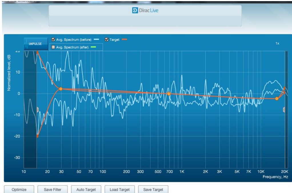
Fig A2-1: Average DIRAC measurement from five different microphone positions in the audience area.
