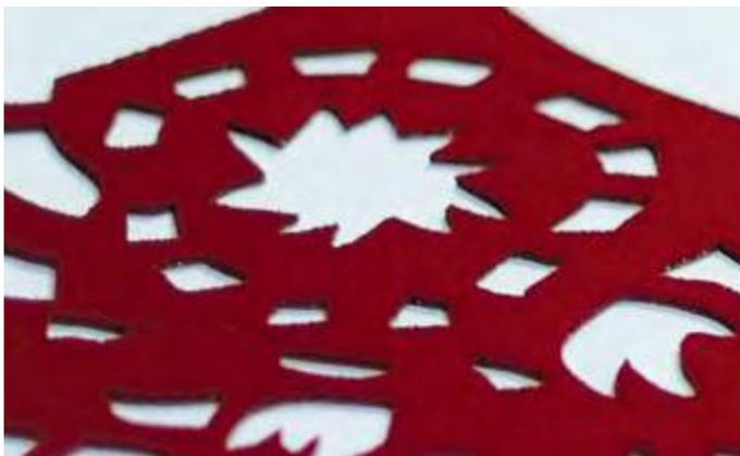
DETAIL OF LASER-CUT RED VELVET, ATTACHED TO A WHITE SATINAC USING DOUBLE-SIDED ADHESIVE TAPE
