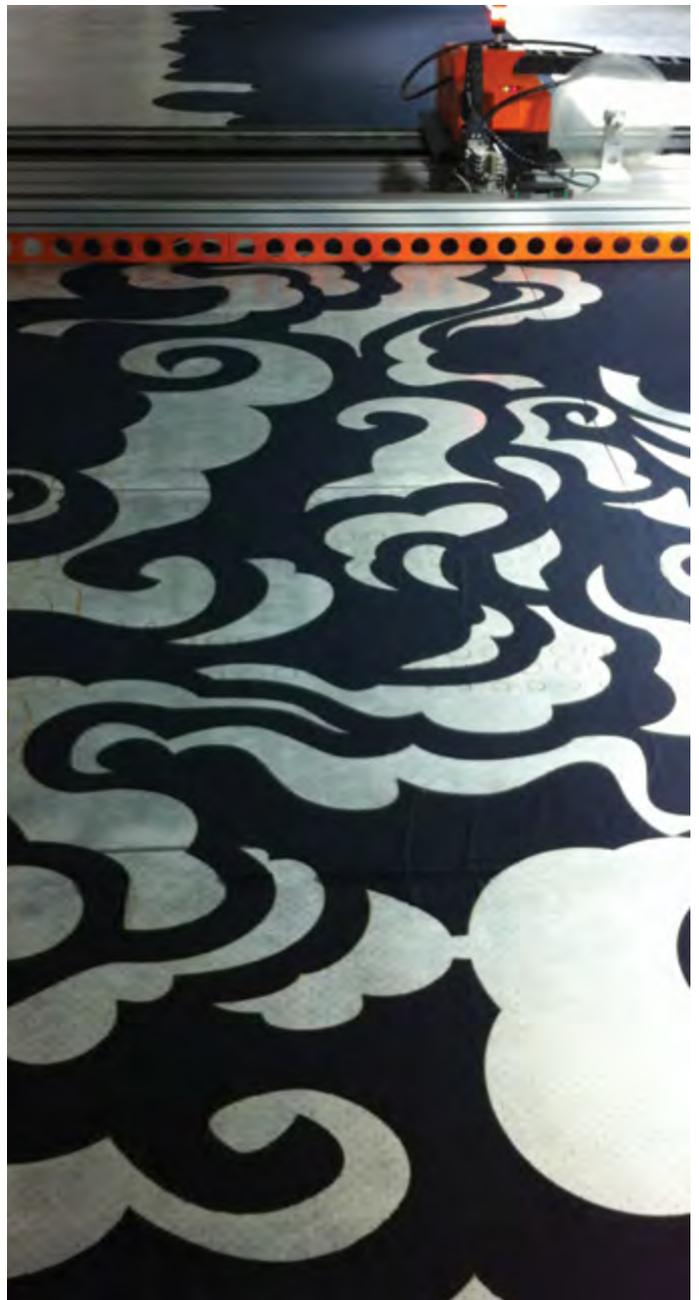
LASER-CUTTING MACHINE CUTTING A BLACK MOLTON CS
