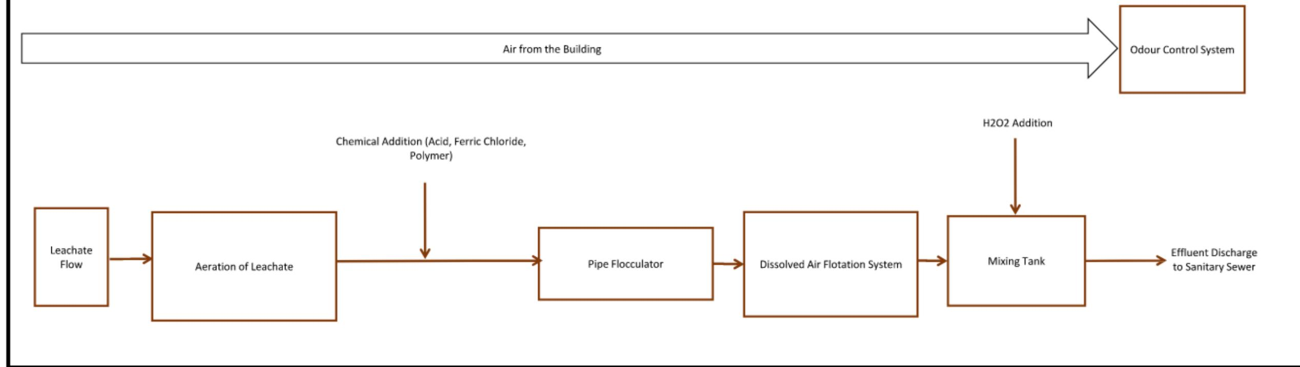
Process Flow Diagram for Long Term Leachate Treatment Process
