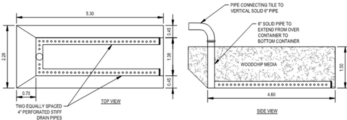
Figure 6 Biofilter Schematic
