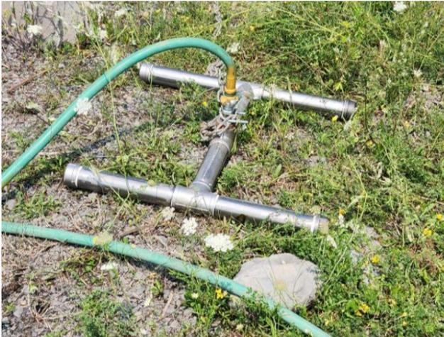
**Figure 4** Coarse Bubble Aerator
