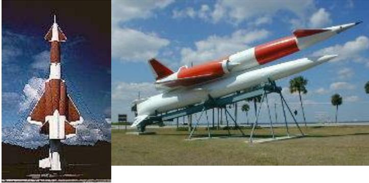
By 1994, corrosion had attacked the fuselage and wings of the Cape Canaveral Museum's XSM-64 (or G-26) Navaho missile. Small plants had taken root in the booster's intertank section. The Navaho was subsequently removed for restoration, returning to a new display site near the Cape's south gate in 1998.
