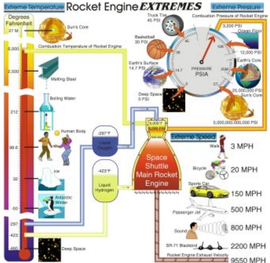
engines and solid rockets reach more than 6,000 degrees Fahrenheit, higher than the boiling point of iron, yet the main engine's fuel, liquid hydrogen, is the second coldest liquid on Earth at minus -423 degrees Fahrenheit.
