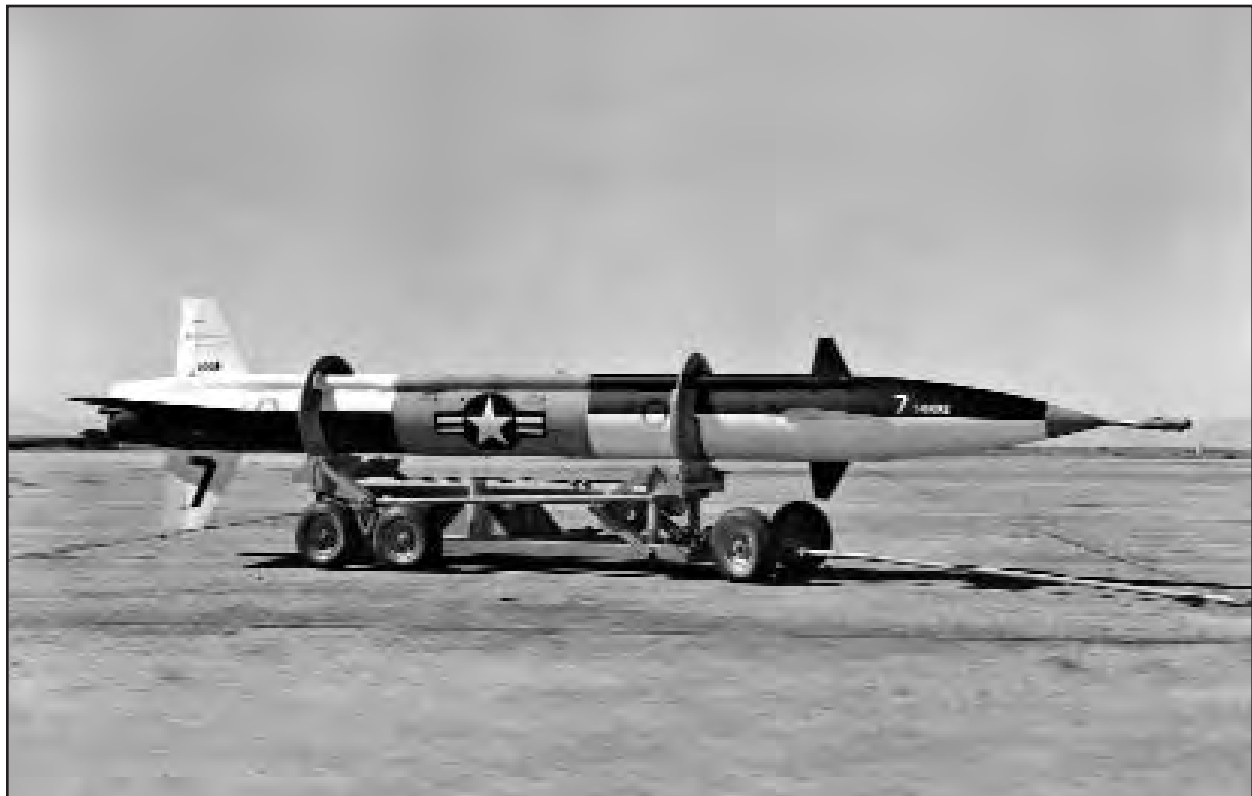
This X-9 was later launched on 16 February 1951 over Holloman AFB, New Mexico, but its flight was cut short by a servo system malfunction. The area around the national insignia was day-glo orange. (Bell Aerospace via the Jay Miller Collection)
