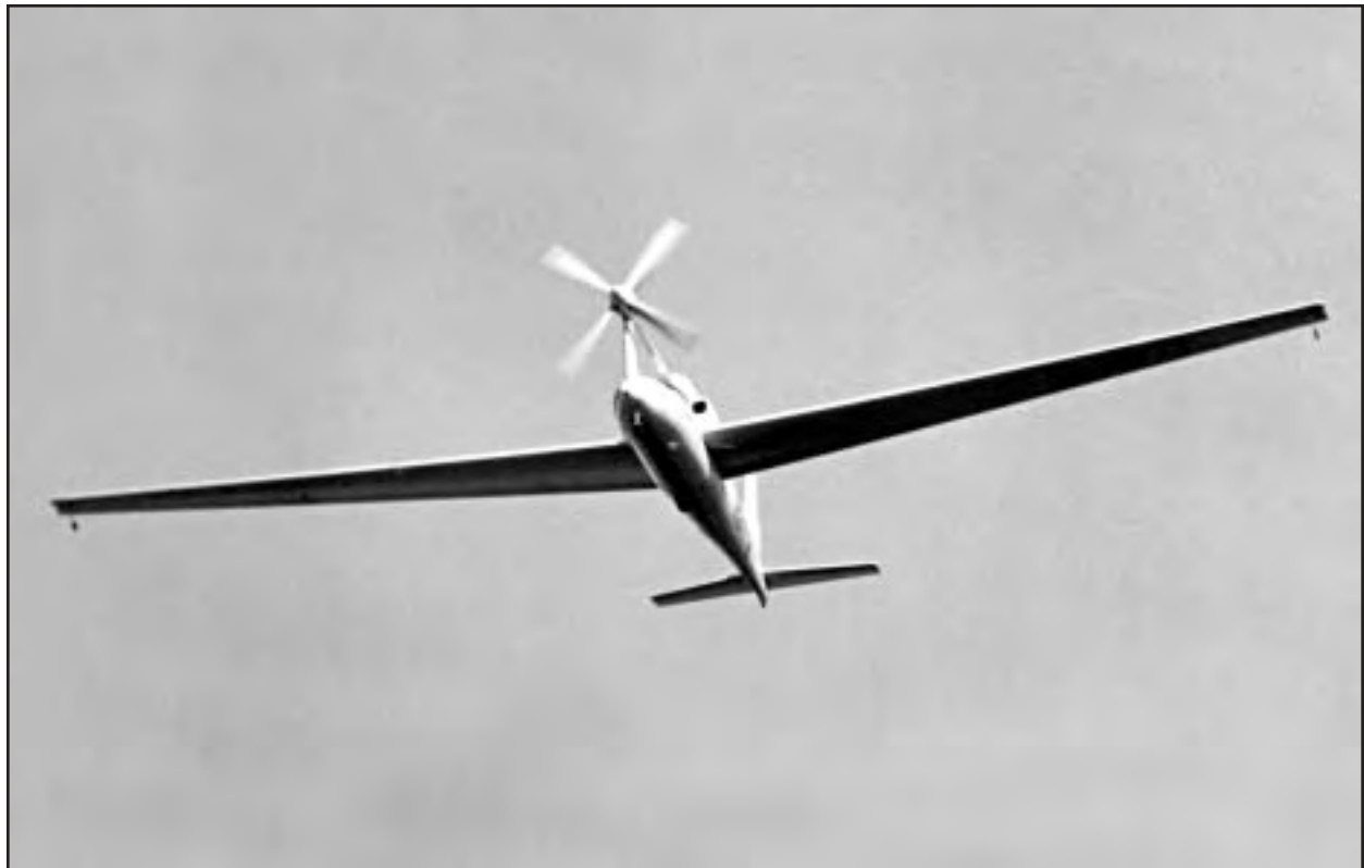
The X-26As were unpowered gliders used by the Navy Test Pilot School. This is an X-26B, a powered derivative used as a stealthy observation aircraft. (Lockheed via the Jay Miller Collection)
