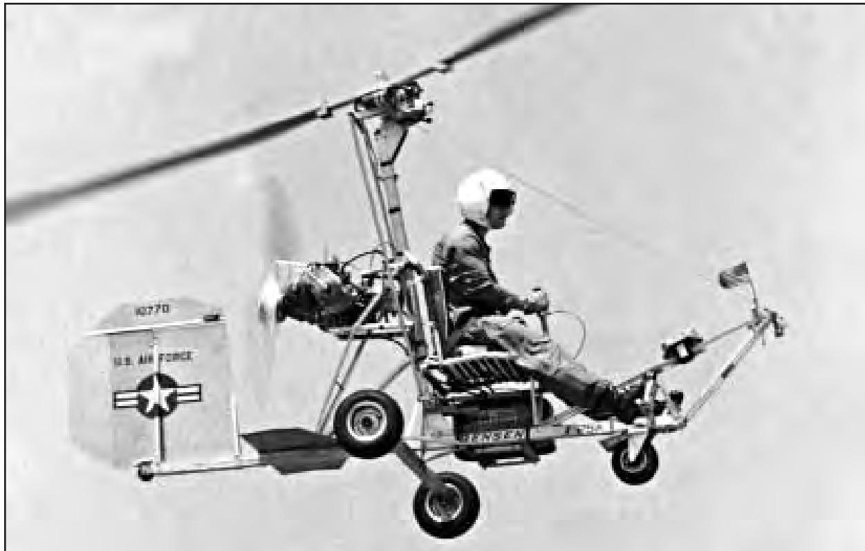
A small 4-cylinder air-cooled McCulloch piston engine mounted directly behind the pilot powered the rotor system of the X-25A. Three different versions of the X-25 were manufactured. (Bensen Aircraft via the Jay Miller Collection)
