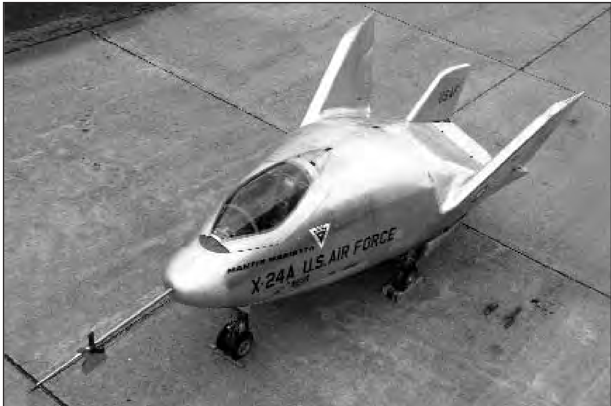
The shape of the X-24A was essentially an enlarged X-23A. Unlike the X-23A, which was designed to explore high-speed flight, the X-24A was designed to explore the low-speed and landing stability of the design. (Martin Marietta via the Jay Miller Collection)
