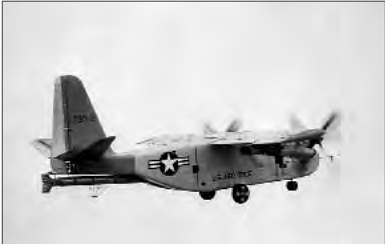
The X-18 was built to investigate the feasibility of a large tilt-wing transport. Unlike the current Bell V-22 Osprey, the entire wing (and the engine assemblies) on the X-18 translated to vertical to support V/STOL flight. (Fairchild via the Jay Miller Collection)
