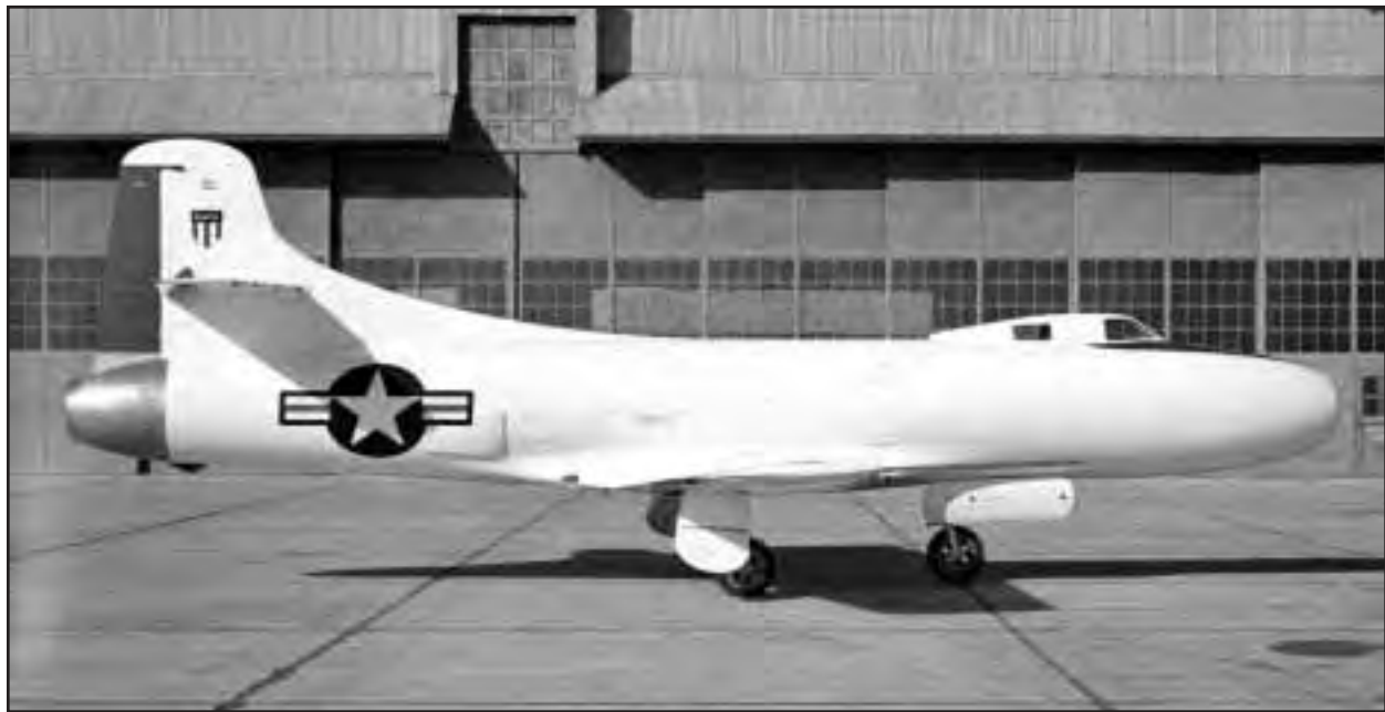
The D-558-I used straight wings and a single turbojet engine—the D-558-II used swept wings and the same Reaction Motors XLR11 that powered the X-1 (and many others). This October 1949 photo shows the Skystreak in its later white paint scheme with an early NACA shield on the vertical stabilizer. (NASA photo E49-090)
