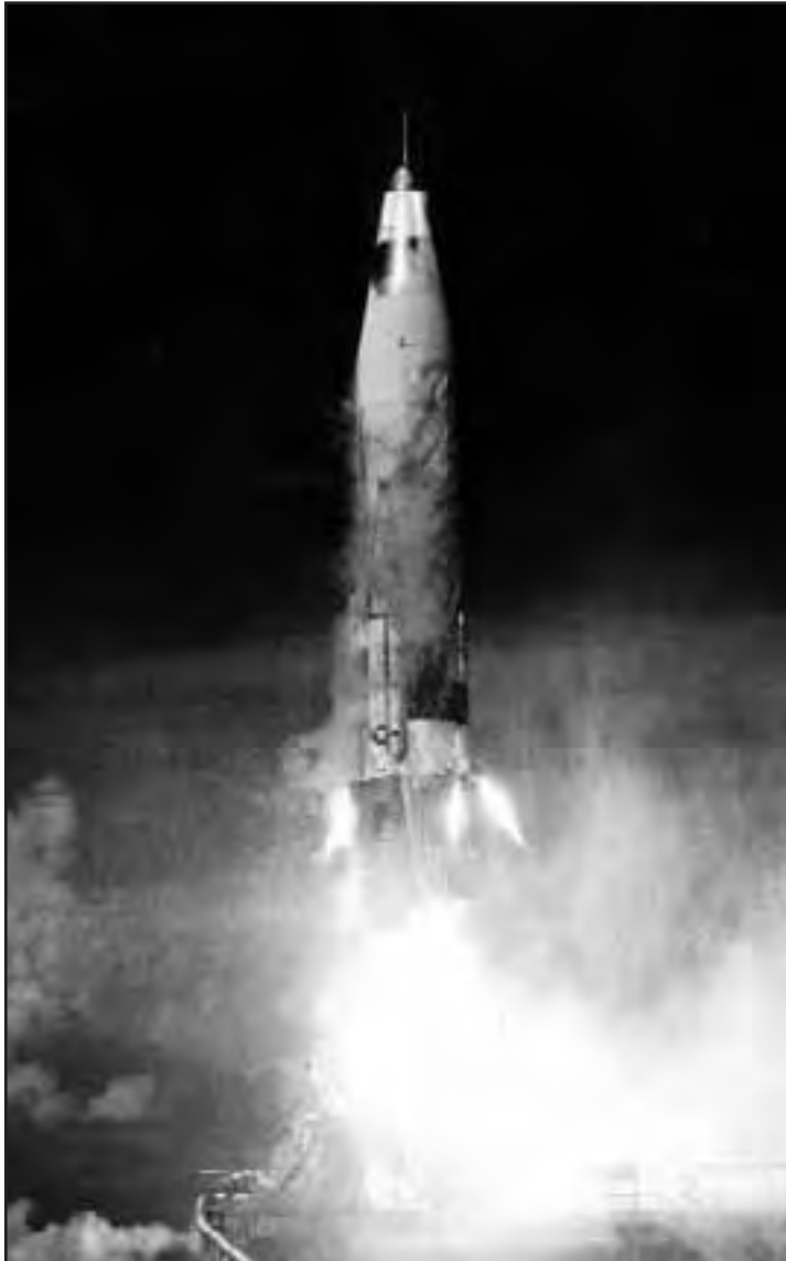
The last Atlas A (vehicle 16A) is launched at Cape Canaveral on 3 June 1958. The Atlas A was an early test version of the three-engine Atlas intercontinental ballistic missile that only used the two booster engines. This was very similar to what the X-11 would have accomplished for the earlier five-engine Atlas design. (USAF/45SW-HO via the Dennis R. Jenkins Collection)
