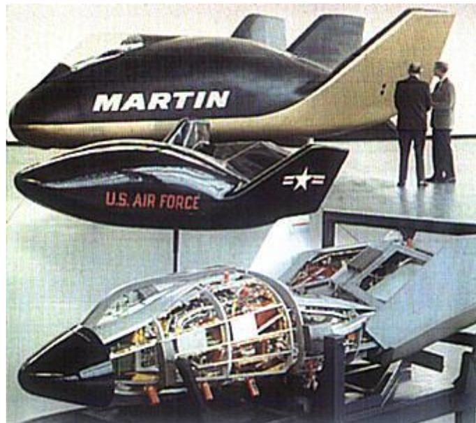
The X-24A was air-launched from an NB-52 carrier aircraft and reached a maximum speed of Mach 1.6 and a maximum altitude of 21,800 m during its flight test. The X-24A handled well as a glider, but in powered flight it exhibited a nose-up trim change that prevented it from flying at low angles of attack. Air Force interest then focused on 'high fineness lifting body' configurations
