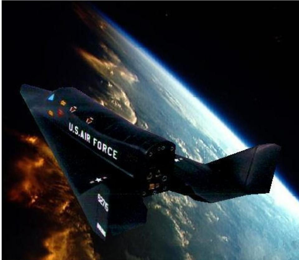
The Dynasoar itself would have been developed into Dynasoar II, III, and Dyna-MOWS (Manned Orbital Weapons System) versions which would have run the gamut of orbital supply, rendezvous and inspection, and orbital bombing. The basic single pilot X-20A Dynasoar had a limited internal payload and volume (450 kg in a payload bay behind the cockpit, enough for another crew member or used for military/scientific payloads).
