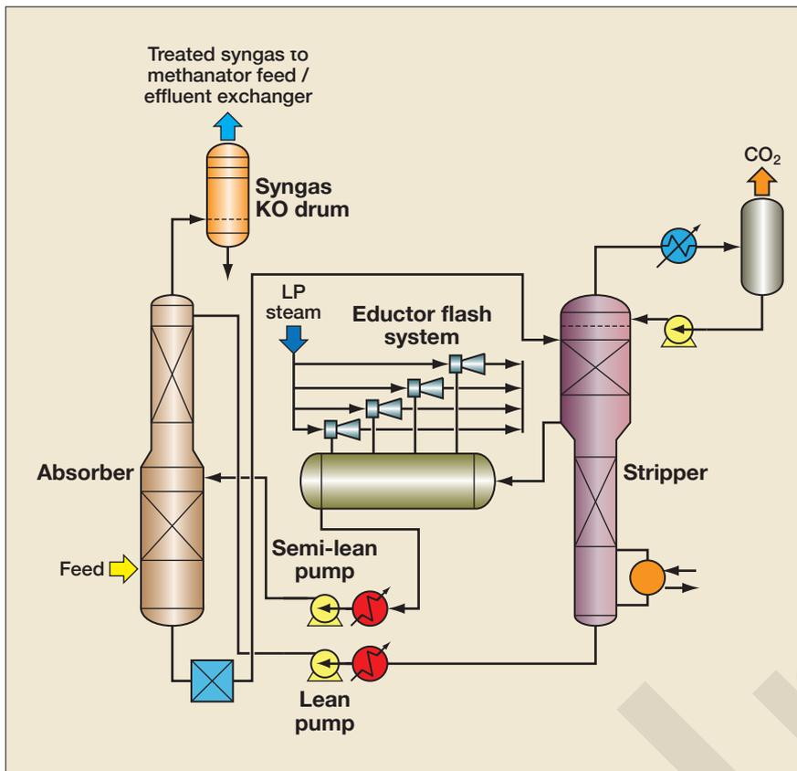
Figure 11 Benfield process schematic for ammonia plants 2 and 3
