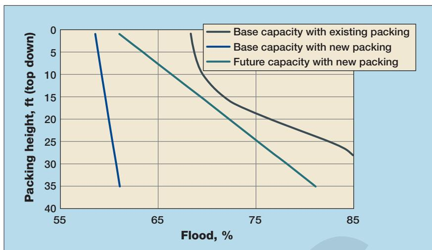
Figure 6 % flood: absorber with new and old packing
