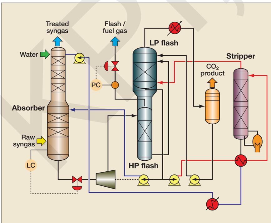
Figure 10 MDEA-piperazine scheme: two stage
