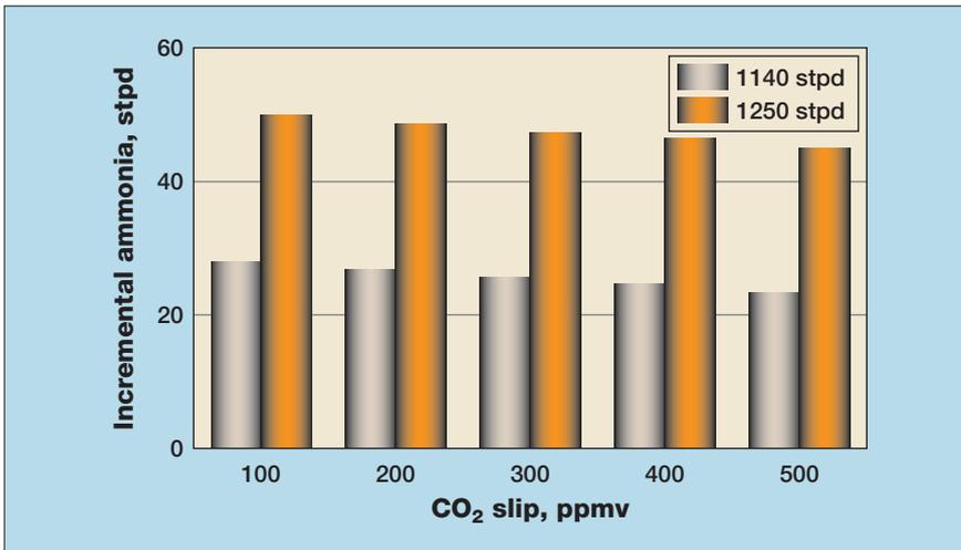
Figure 8 Incremental ammonia production with reduced CO<sub>2</sub> slip
