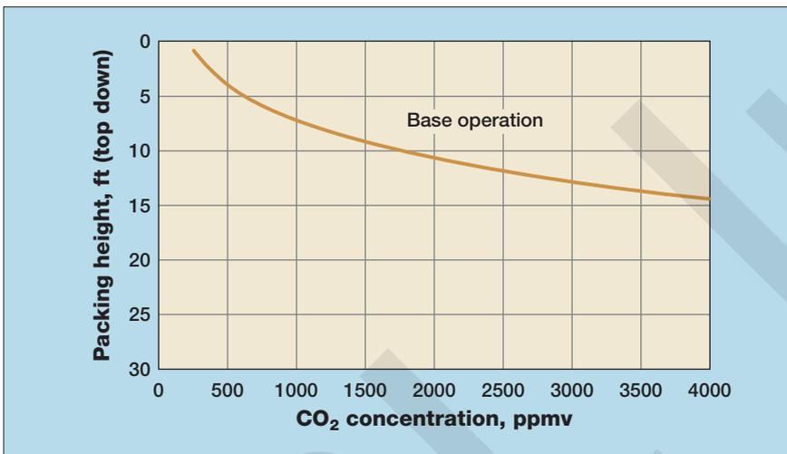
Figure 4 Absorber vapour CO<sub>2</sub> concentration profile
