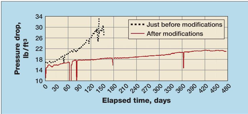
Figure 12  $\Delta P$  trend before and after modifications
