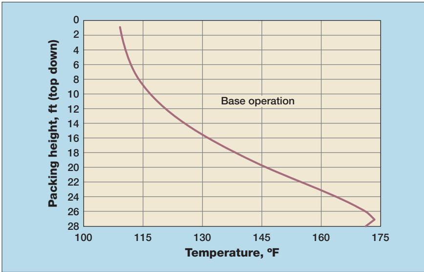
Figure 3 Absorber temperature profile
