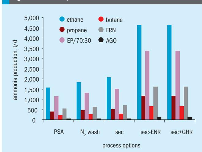
Fig 7b: Ammonia production from methanol, CO and PDH plants
