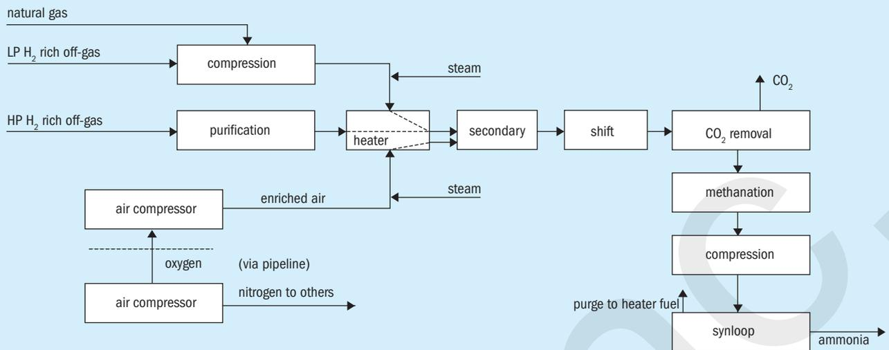
Fig 6: Secondary reforming with GHR option
