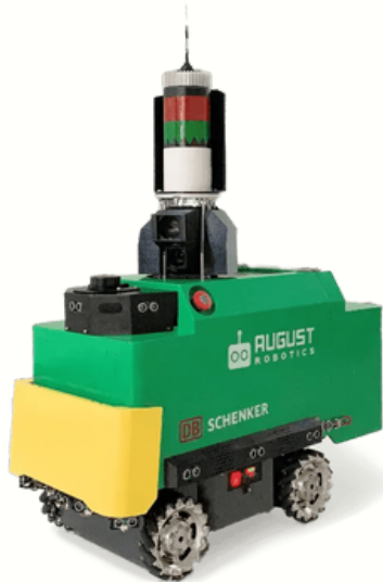
Lionel Exhibition floor marking robot
