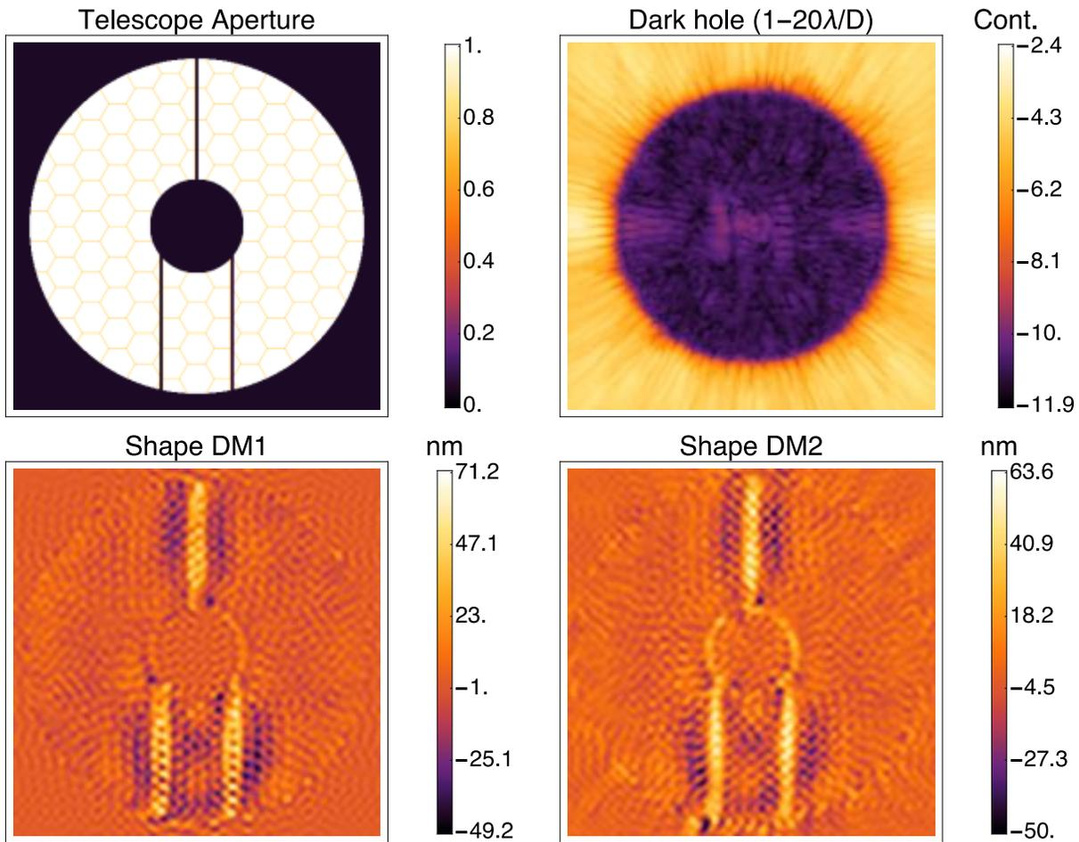
**Figure 3:** Coronagraph design for the *LUVOIR* Architecture "A" based on a Vector Vortex focal plane mask and using the ACAD-OSM technique to control the DMs. Courtesy of J. Mazoyer.
