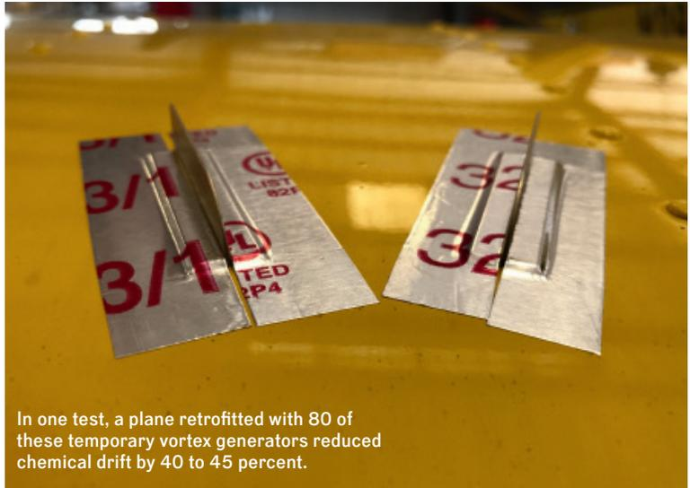
In one test, a plane retrofitted with 80 of these temporary vortex generators reduced chemical drift by 40 to 45 percent.
