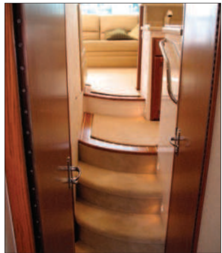
Above —The companionway of this 29-footer (8.8m) is too narrow; and the folding hatch interferes with the view from the helm. Above right —These steps are unevenly spaced and too steep, making access to the cabin unnecessarily hazardous. Right —The Cabo 40 (12.3m) has near-perfect home-like stairs with easy risers and a well-placed handrail.
