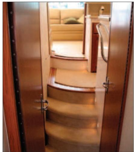
Probably the most important location is at the companionway's long drop from the bridge deck to the base of the ladder. Grabrails are also important around the galley, so you won't lose your balance or fall against a hot stovetop or oven.
