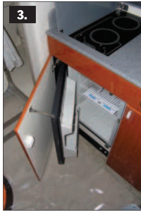
1 —The compact galley aboard a Back Cove 29 (8.8m). It includes a proportionally large countertop, with work space between the sink and recessed stove. 2 —The True North 38 (11.5m) has a galley-up arrangement with generous work space and ventilation. 3 —Details on the Formula 31 PC (9.6m) include a clever door-on-door for the fridge, and a switch that shuts off power when the stove lid closes. 4 —The Tiara 3900 (11.8m) Sovran's galley is also a great work space thanks to natural light, a toe kick even at the unusual central sink installation, and a grabrail.
