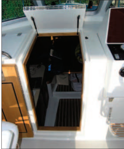
Above —The companionway of this 29-footer (8.8m) is too narrow; and the folding hatch interferes with the view from the helm. Above right —These steps are unevenly spaced and too steep, making access to the cabin unnecessarily hazardous. Right —The Cabo 40 (12.3m) has near-perfect home-like stairs with easy risers and a well-placed handrail.
