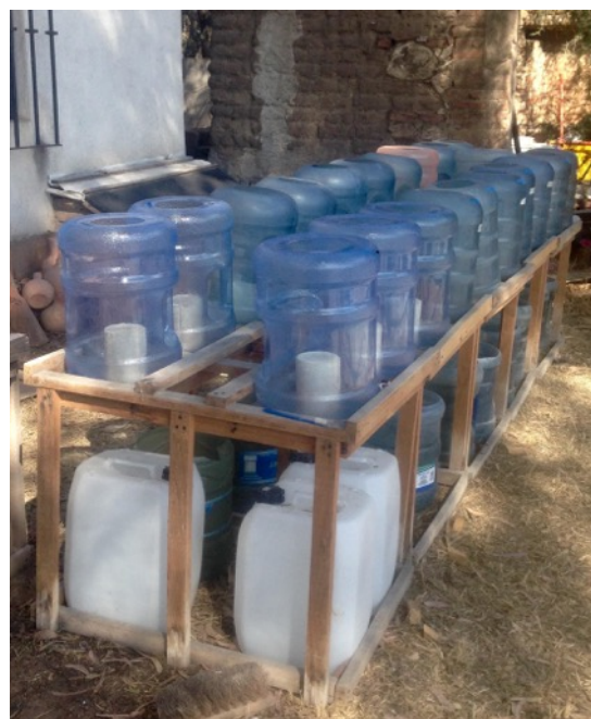
Used filter systems set-up for flow and biological testing.
