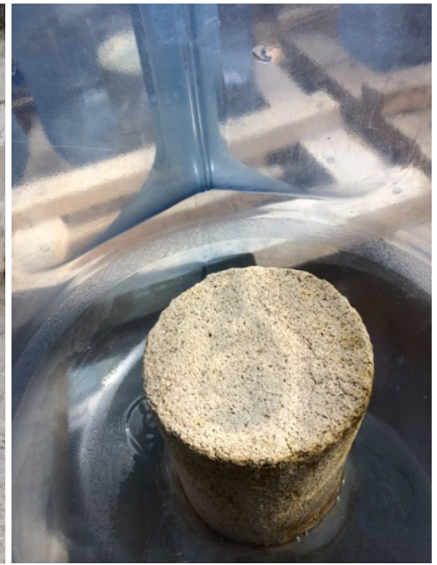
Top Right: Kids come to change out used filter system in Juan Gonzalez; Top Left: Ceramic filter after 3.5 years of use. Discoloration and some physical degradation is visible.
