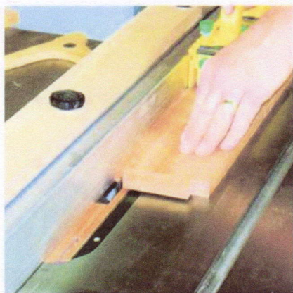
Using his table saw with a 1/4" dado head, the author plows grooves that will capture and secure the sub-top.
