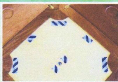
Double-sided carpet tape is used to secure the felt playing field to the frame subassembly. Use several pieces, as shown above.
