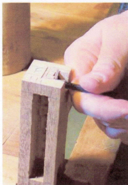
The top stretcher is joined to the leg using a dovetail rather than a mortise. The author formed the tail on the stretcher first, then transferred the shape to the top of the leg.
