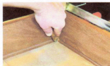
The sub-top is made from good quality plywood. The author forms a tongue around the edge of the sub-top using a dado head in his table saw.
