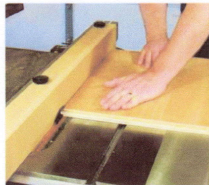
The sub-top is made from good quality plywood. The author forms a tongue around the edge of the sub-top using a dado head in his table saw.
