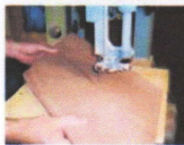
Using your template, mark out four leaves for the table. The author recommends that all four pieces come from the same piece of stock.
