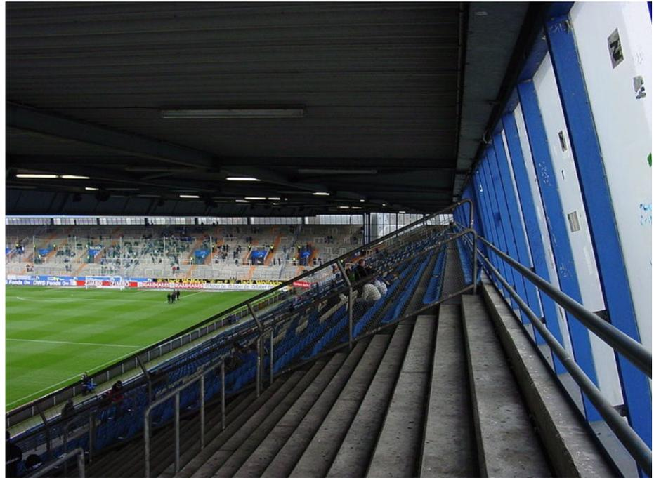
Figure 2: Regular terraces, to be fitted with clip-on seats for UEFA and international games
