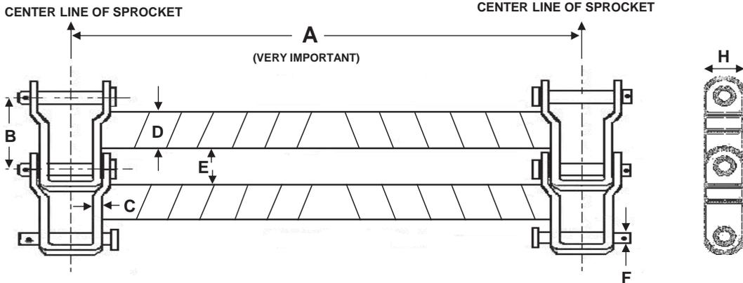
(A) SPROCKET - CENTER LINE TO CENTER LINE = \_\_\_\_\_ (IN INCHES)
