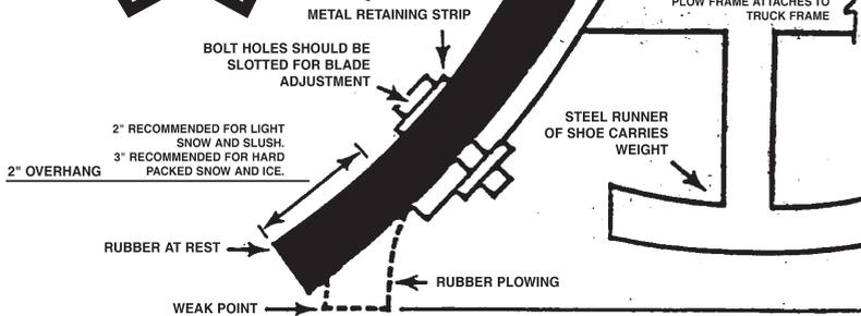
Rubber blades will not damage brick streets, curbs, manhole covers, speed bumps, reflectors, etc...
