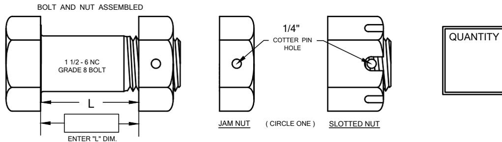
THE "L" DIMENSION IS THE REQUIRED DISTANCE BETWEEN THE BOLT HEAD AND NUT WHEN ASSEMBLED ON THE BLADE AND BLADE BAR. THIS DIMENSION DETERMINES THE BOLT TO BE USED TO ATTAIN THE MAXIMUM SHOULDER LENGTH FOR BEST WEAR RESISTANCE. NO OTHER DIMENSIONS ARE NECESSARY.
