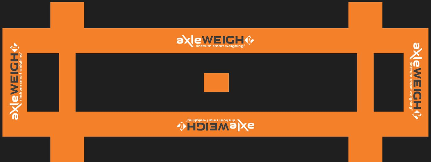
Drive over the scale at a constant speed ~3MPH | ~5km/h
