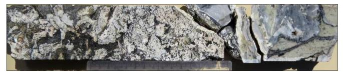
Figure 13. Felsic dyke with sphalerite, galena and fine visible gold (IDH006 at 78.0m).
