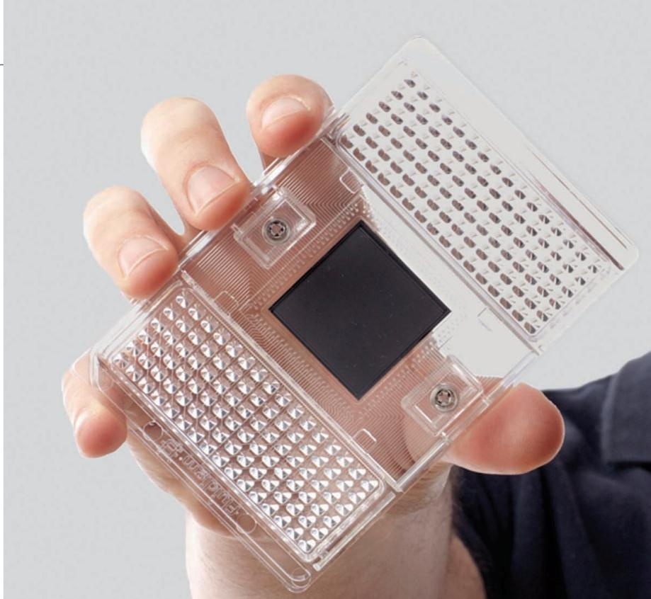
**Convergence at work.** Microfabricated device by Stephen Quake, Stanford University, for sequencing DNA from one sperm.
