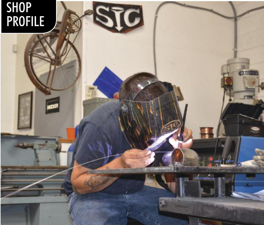
The shop's fabricator Noel Castillo is shown TIG-welding a three-inch stainless steel exhaust.
