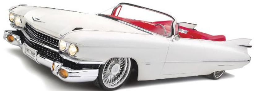
The 1959 Caddy built by SIC Chops for Rich Tillema features a one-off Roadster Shop chassis, one-off Colorado Custom wheels, and a 650-hp Cadillac CTS-V LSA power plant with a 6L80 transmission. Other features include air ride by AccuAir and a custom Ron Mangus red leather interior. (Photo by RoddingRevolutions.com)
