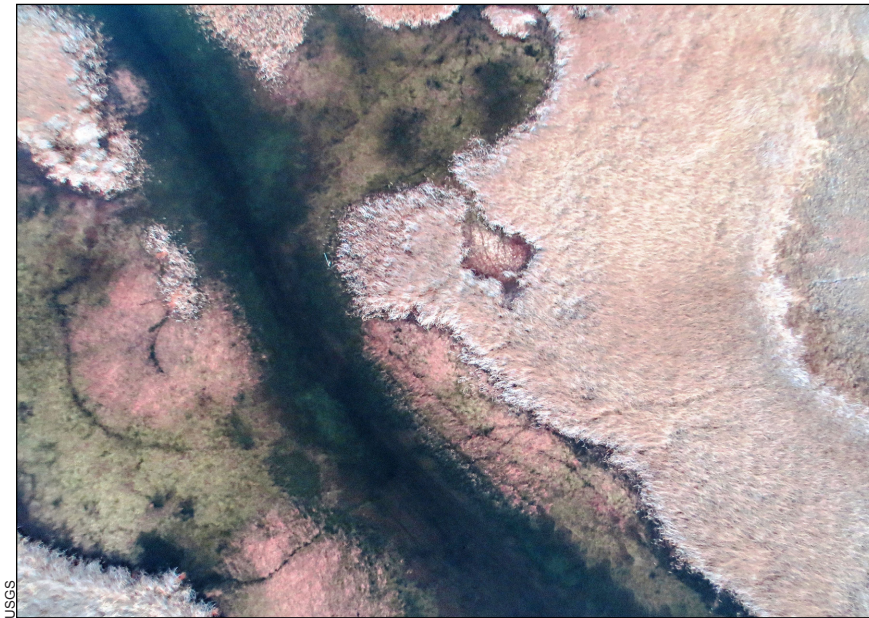
Figure 5. A color infrared (IR) image of wetland vegetation used to identify habitat for US federally listed wetland birds. Color IR images were used to generate NDVI values, which in turn were used to classify habitat types.
