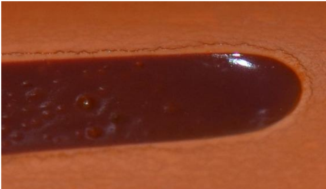
Figure 1. Incipient ESC cracking is apparent as a halo around the perimeter of a cement drip.
