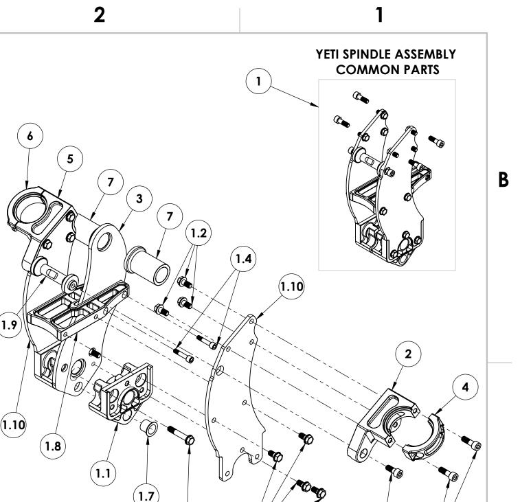
2017 SPINDLE ASSEMBLY, 35MM OFFSET, 48MM DROP, 48MM FORK, 190MM CL
