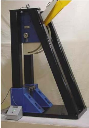
The MPM Charpy/Izod 9000 Series impact test machines can be used with pendulums in the 100 ft-lb to 700 ft-lb energy capacity range. The various energy capacities are achieved by changing the pendulum. Since the machine frame has been designed for up to 700 ft-lbs, any lower capacity can be accommodated. Therefore, you can upgrade your machine capacity later by purchasing a higher capacity pendulum without the need to buy an entire test machine.
