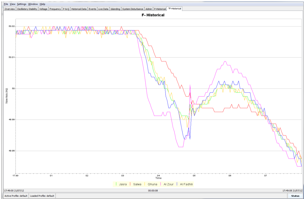
Figure 15 – System Frequency Information for a Generator Trip
