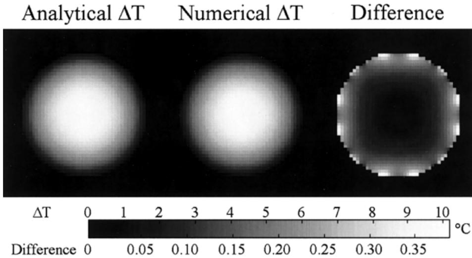
**Figure 1.** Analytically (left) and numerically (center) calculated increase in temperature ( $\Delta T$ ) distributions for the sphere of unperfused brain tissue after application of uniform SAR of 3.0 W/kg, and the difference (right) of the numerically calculated value from the analytically calculated value. Grayscale values are given in  $^{\circ}\text{C}$ .
