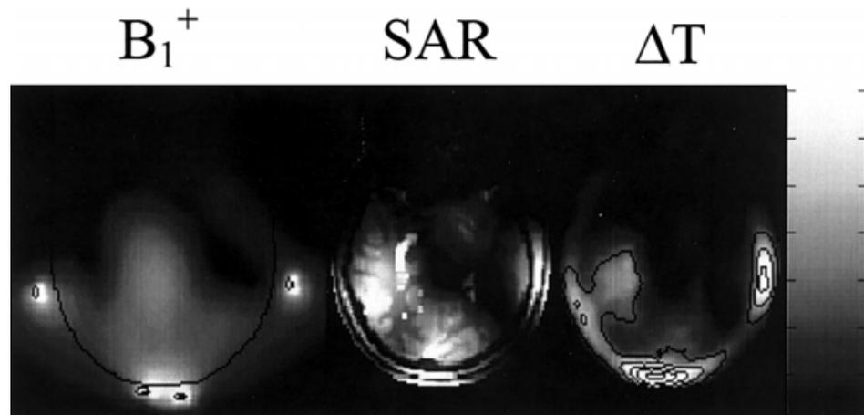
**Figure 3.** Distributions of  $B_1^+$  (left), SAR (center), and resulting temperature increase (right) for quadrature surface coil at 300 MHz. Linear grayscale is from 0 (black) to 15 mT (white) for  $B_1^+$ , 0 to 20 W/kg for SAR, and 0 to 1.5°C for temperature increase. Contours for temperature increase at 0.5, 1, 1.5, 2.0, and 2.5°C.
