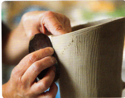
2 Scraping the pot with a surform blade and then a metal kidney.
