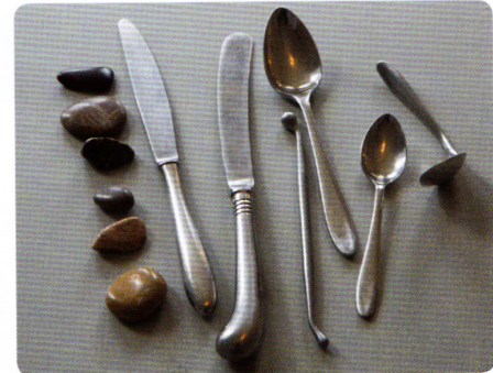
6 Burnishing tools: different tools are used to burnish different parts of the pot.
