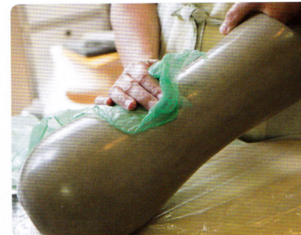
10 Final polishing with a plastic bag. The pot is left to dry, and then fired to 920°C.
