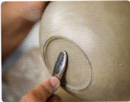
7 Burnishing the base with the handle of a metal spoon. Get into the nooks and crannies with a 'bone' tool.
