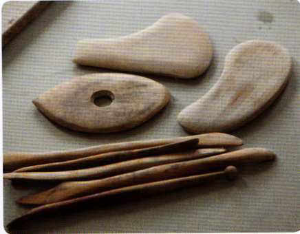
4 Wooden ribs and tools used for smoothing the surface of the pot.
