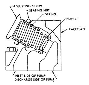
The relief valve must be positioned as shown in instructions for direction of rotation — otherwise the valve is inoperable and will not give protection.
