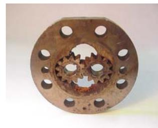
*Gears fused to corroded case*
