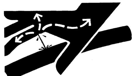
**Injection Hazard: Do not try to stop a leak with your hand! Avoid any close contact with hydraulic fluid jets. Escaping fluid can penetrate skin, causing serious injury. In case of accident, see a doctor immediately for removal of fluid.**
