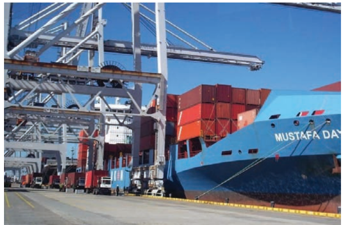
Figure 2.6: Jockey trucks preparing to unload in the marshalling area
