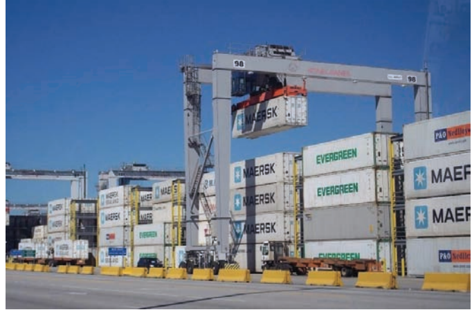
Figure 2.5: A rubber-tired gantry crane moves a forty foot container in the container field
