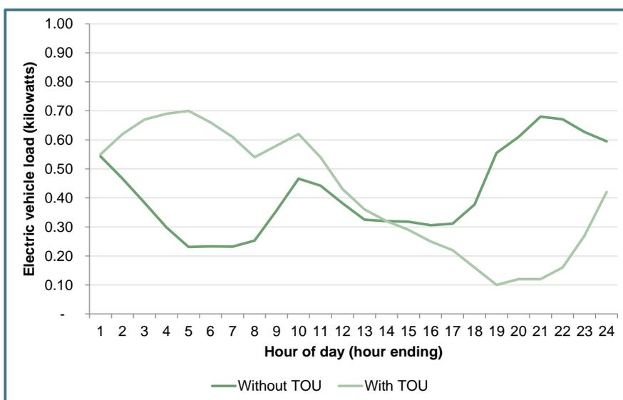
**Figure 11: Electric vehicle charging patterns with and without TOU rates and workplace charging**
