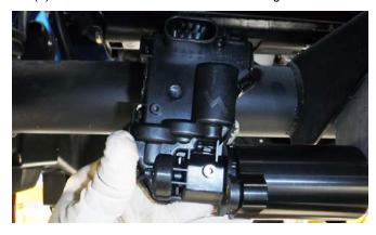
Connect supplied wire harness to actuator. Then connect
