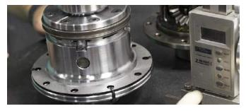
Measure the difference between the new and original Ring Gear Flange height. Identify and record the difference between the two heights.
