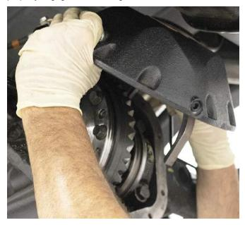
Apply a generous bead of the supplied RTV sealer to axle housing
