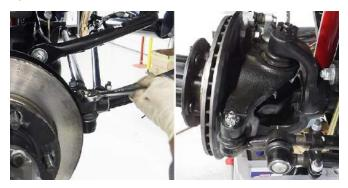
14. Install front wheel and tire and torque to specifications.
