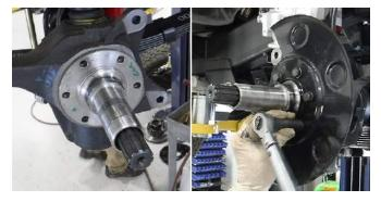
Install hub and rotor assembly, then install (1) inner spindle nut, (1) toothed lock washer and (1) outer spindle nut and torque to specifications. Bend at least one tab on the toothed lock washer.
