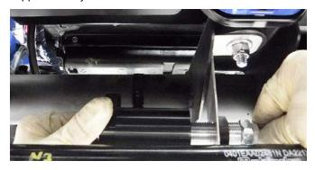
Apply none drying lubricant to the OX locker actuator cable (long barrel end), install the threaded sleeve and tighten cable length jam nut.
