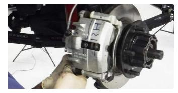
12. Slide the axle forward slightly and install the snap ring.
