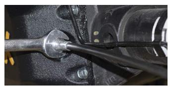
8. Install (10) 12 mm differential cover bolts and torque to specifications.
