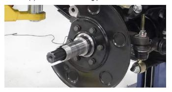
12. Remove wheel bearing spindle.
