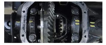
Rotate the differential into a position to pry on the casting.
