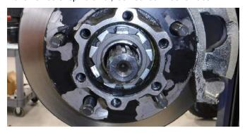
Remove (1) outer spindle nut, (1) toothed lock washer and (1) inner spindle nut with a 50 mm socket.
