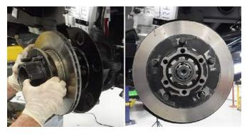
11. Install brake caliper mounting bracket bolts using a 19 mm socket and torque to specifications.
