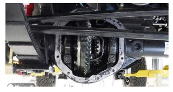
Mark differential bearing caps so they can be reinstalled in their original orientation, then remove (4) bearing cap bolts with a 19 mm socket.
