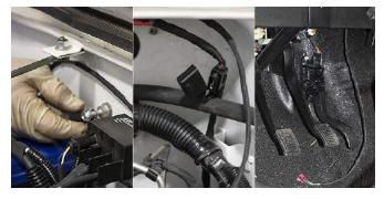
9. Remove the Deutsch connecter from the Ignition Switch and install the red power wire into the position shown.
