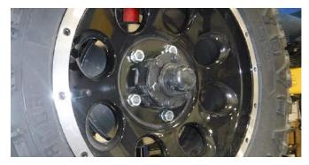
4. Remove (1) hub dust cap using two pry bars, then remove (1) outer axle shaft snap ring using snap ring pliers.
