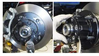
6. Flatten all outer spindle nut, toothed lock washer tabs.
