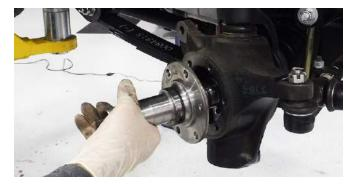
Pull front axle shaft assembly out until you feel it disengage the differential.
