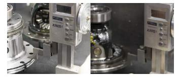
3. Add or subtract shims to the Driver's side of the carrier until the two heights are identical.
