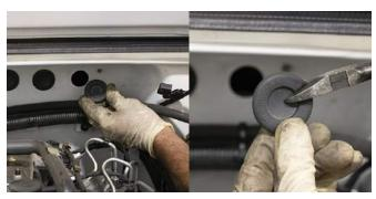
Connect harness ground to ground stub near battery. Then
