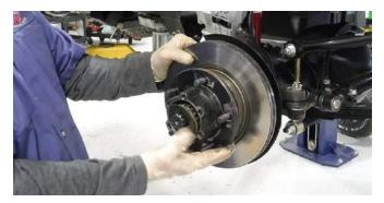
11. Remove (6) 14 mm brake backing plate bolts.
