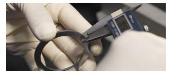
4. Measure the difference between the overall height of the new Front Axle Carrier and original. Identify and record the difference between the two heights.
