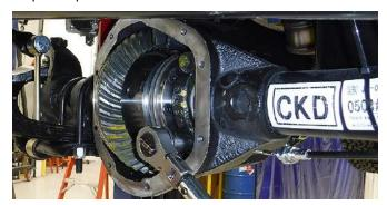
2. Check to ensure that backlash is between .005" - .010" (.13 mm - .25 mm)
