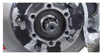
8. Remove the master tie rod assembly cotter pin and castle nut with a 19 mm socket. Separate and secure it forward out of the way of the differential cover.
