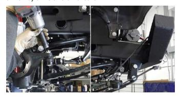
Remove (2) brake caliper mounting bracket bolts using a 19 mm socket and hang out of the way.
