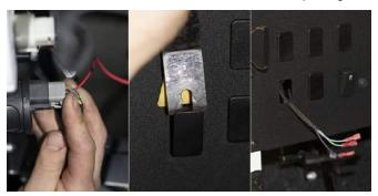
11. Reinstall the inline fuse. Connect the OX Locker Switch to the harness following the color scheme listed on the switch, then install switch to dash panel. Power on the Ignition Key and verify the Electric Actuator is working. The switch will light up when the OX Locker is engaged. If
