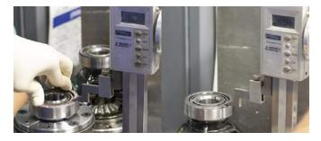
Add or subtract shims to the Passengers side of the carrier until the two heights are identical.
