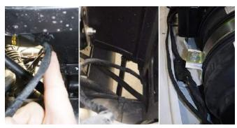
7. Remove one of the bulkhead grommets and install a slit/ hole to route wire harness thru.
