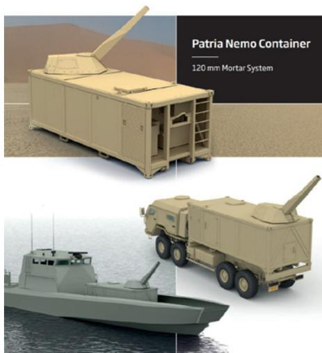
The customer can select NBC (Nuclear, Biological and Chemical) filtration systems, as well as the desired ballistic protection, made either of steel plates or ceramic armour. High-durability steel plating 8 to 10 mm thick adds around three tons to the weight of the container.
