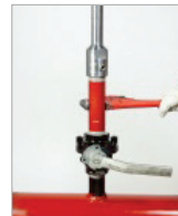
Figure 4.65. Unscrew Drilling Machine
