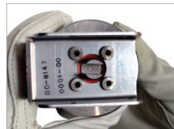
Figure 7.3. Push Rod and Screws Installed
