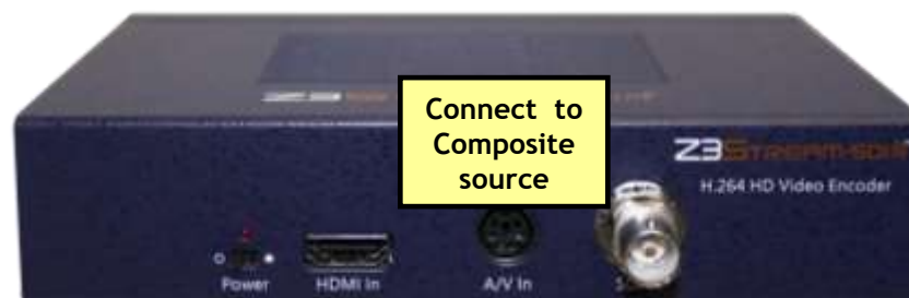
Figure 12 Composite Connection for Encoding
