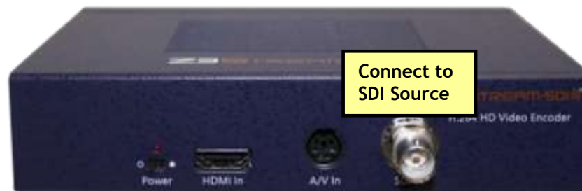
Figure 7 SDI Connection for Encoding
