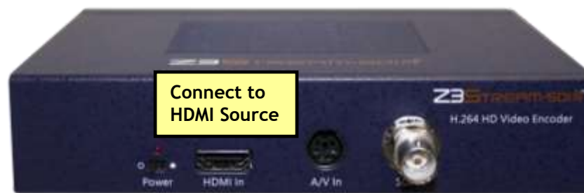
Figure 9 HDMI Connection for Encoding
