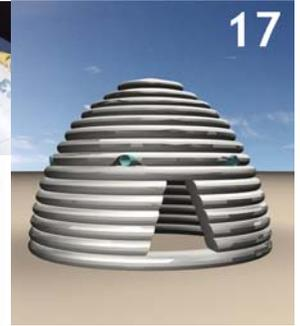
**14, 15) You must use 2 Compasses to make the dome shape. Use chains or other non-stretchy cable-ropes. Attach one in the center (Center Compass), and extend the length at every row according to a second one at the perimeter (Height Compass). If any bags do not conform to the compass remove them and re-build.**
