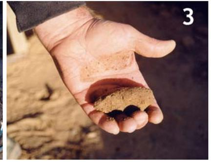
1) Collect the tools above. 2) Prepare the earth mix which is stabilized with cement or lime, or asphalt emulsion. 3) Add enough water to ball together when squeezed, yet not leave the hand wet. If no cement/lime is available, use raw earth for a temporary shelter. (Experimental - try snow in bags and compact.)
