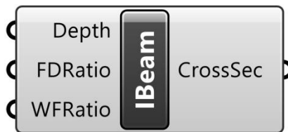
Figure 57 – The I-Beam (IBeam) component
