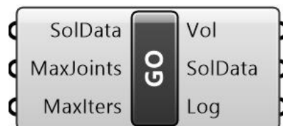
Figure 66 – The Geometry Optimization (GO) component
