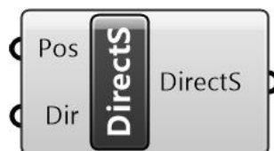
Figure 38 – The Directional Support (DirectionS) component
