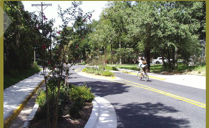
Chicane, Source: nacto.org/publication/urban-street-design-guide/street-design-elements/curb-extensions/chicane/
