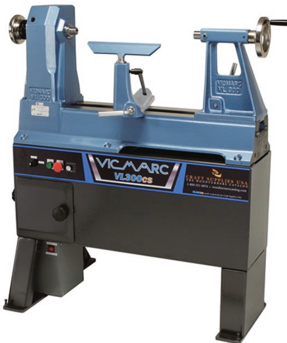
Vicmarc - Large swing lathes are attractive to bowl turners, and these lathes are also offered in long bed versions
