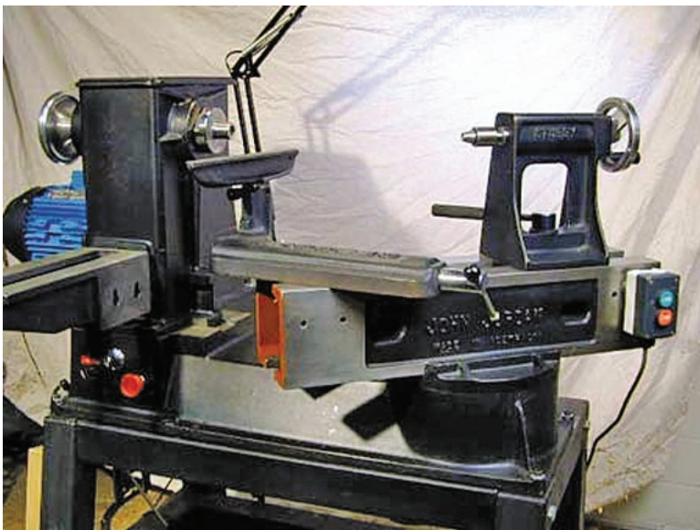
Stubby - Innovative design allows the bed to be rotated at any angle to the axis
