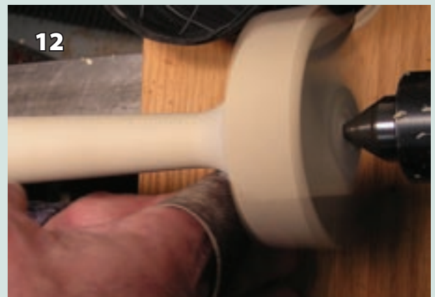
Light pressure and patience are required to carefully sand the intermittent part at the top of the foot.
