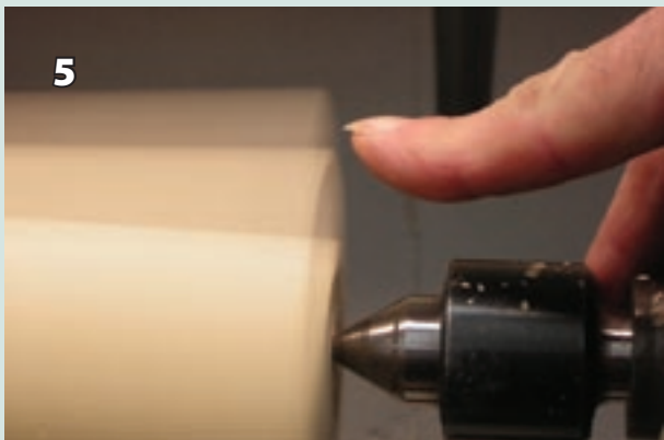
5 Rough out to \frac{1}{8} " above the second shadow line as pointed out by my fingernail.
