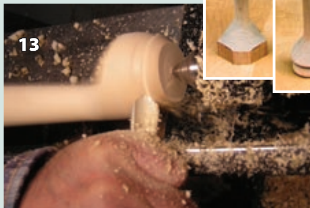
Use a \frac{1}{2} " spindle gouge to round the bottom of the foot. The curve begins just above the point of the toe.
