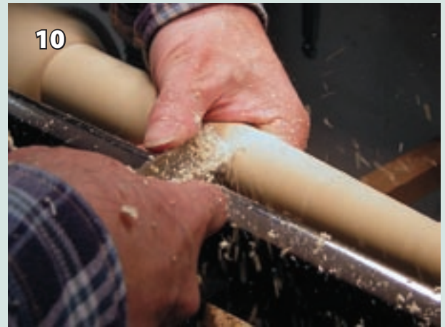
A shallow spindle gouge is used for final finishing. The left hand dampens vibrations and can detect errors that the eye cannot.
