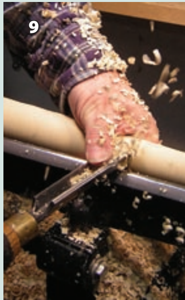
A \frac{3}{4} " roughing gouge is used first to taper the leg. The left hand is used to dampen workpiece vibration. The gouge is guided by the thumb.
