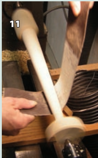
A broken sanding belt works well on straight tapers.
