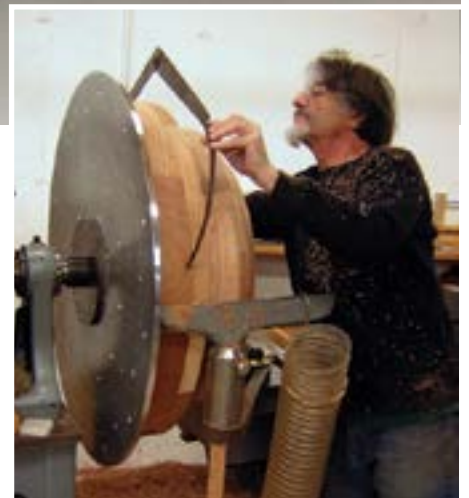
Jon measuring a replacement column base for an historic building
