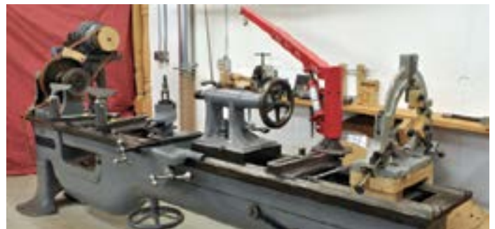
Jon’s heavy-duty Putnam pattern maker’s lathe, from about 1900. This style is called an ‘extension bed lathe’ and the bed has separate upper and lower tiers
