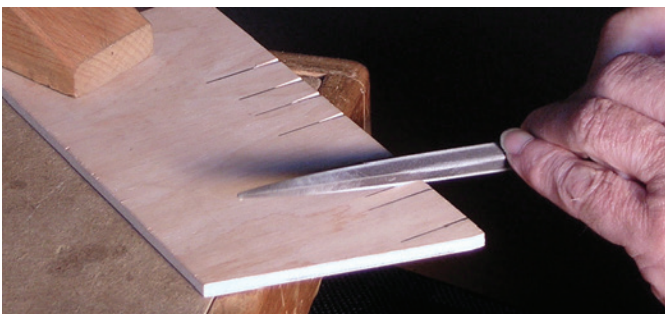
9 Filing notches in marking board—Use a triangular file to make notches in the marking board parallel to the grain of the top veneer.
