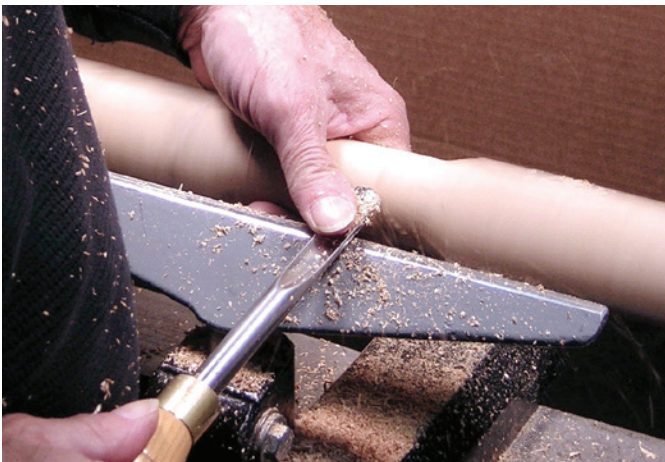
5 Preparation for steady rest—The area where the steady rest is to be placed must be smooth and totally free from chatter marks.
