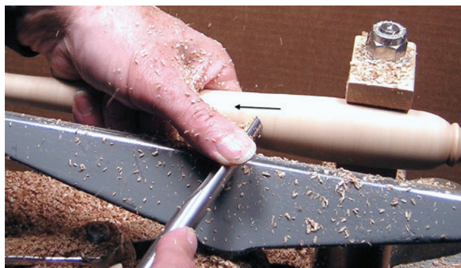
14 For finishing, the spindle gouge is used with a shearing “pull cut”, which means that the handle is ahead of the cutting edge.
