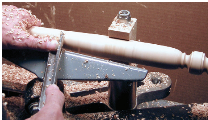
13 Material is removed quickly with \frac{3}{4} " spindle roughing gouge.
