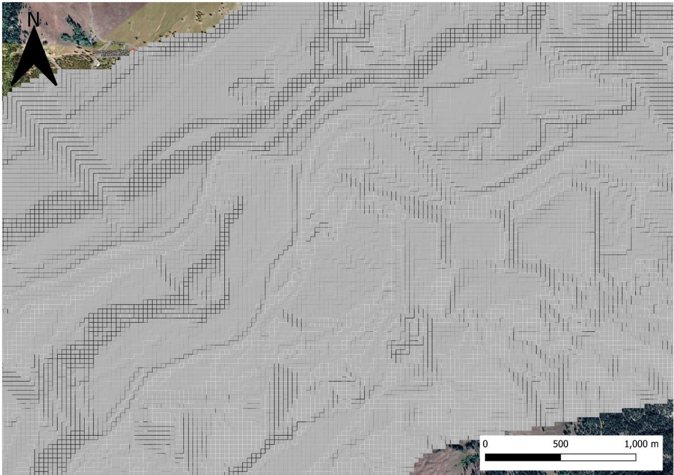
*A 21: Hillshade rendering of the 30 m interpolation of the DEM used in the FLO-2D simulations with the 30 m model domain. The raw underlying DEM includes both the 1 m lidar DEM and the 10 m NHDPlus-HR DEM, where needed. An example of the seam between these two datasets can be seen in the NE corner of the hillshade image (NE-SW trending line).*
