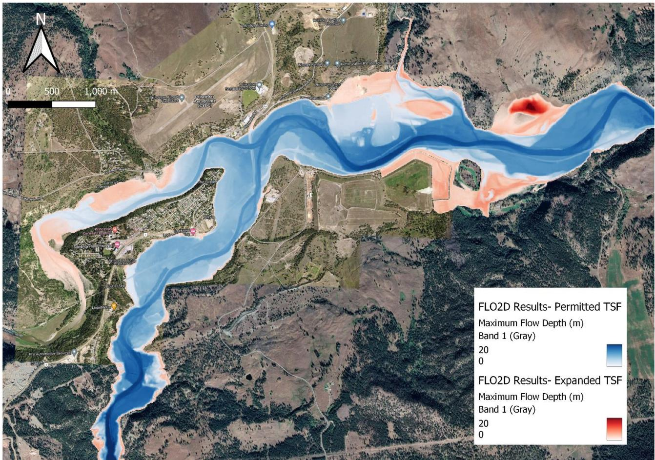
**Figure 5-1: An overlay of maximum flow depths (m) in Princeton, BC from a 40% breach, 12 hour duration scenario for the permitted TSF (250 Mm<sup>3</sup>; in blue colorbar) and the expanded TSF (450 Mm<sup>3</sup>; in red colorbar)**
