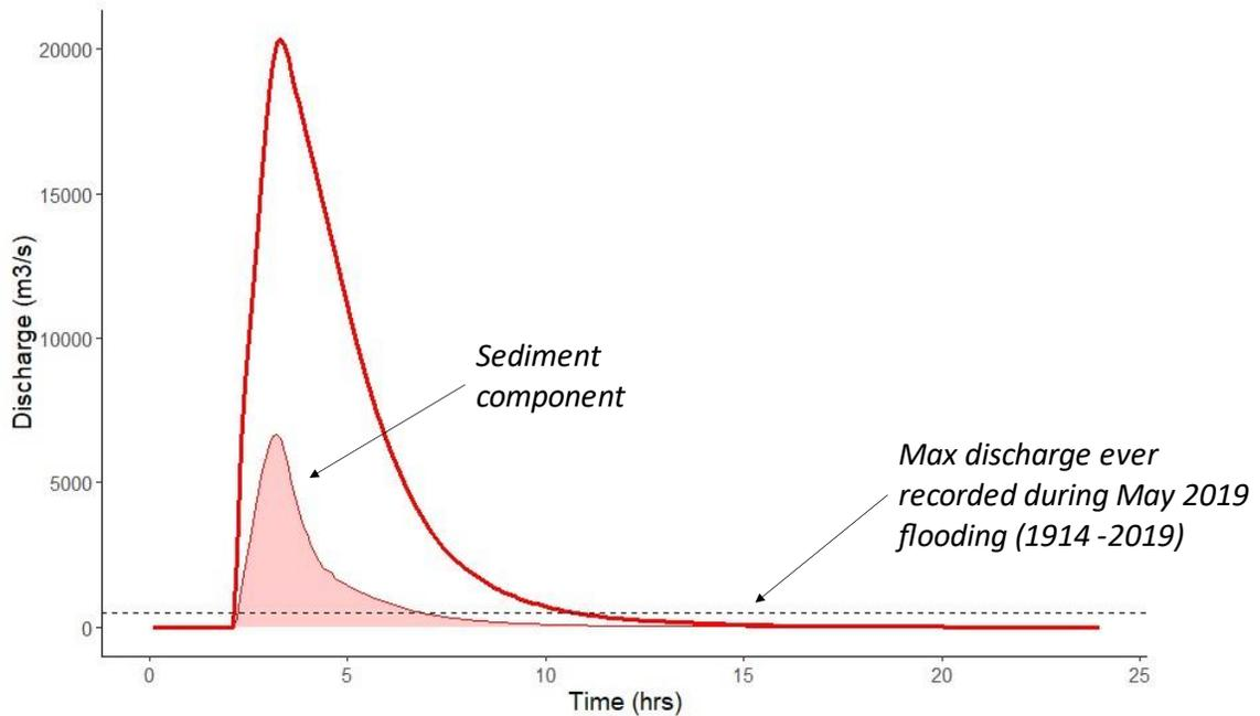
**Figure 4-7: Timeseries hydrograph of the first 24 hours of the default expanded dam breach scenario. The bulked component (dark red line) is 12 times more than the maximum discharge ever recorded at gage 08NL007.**
