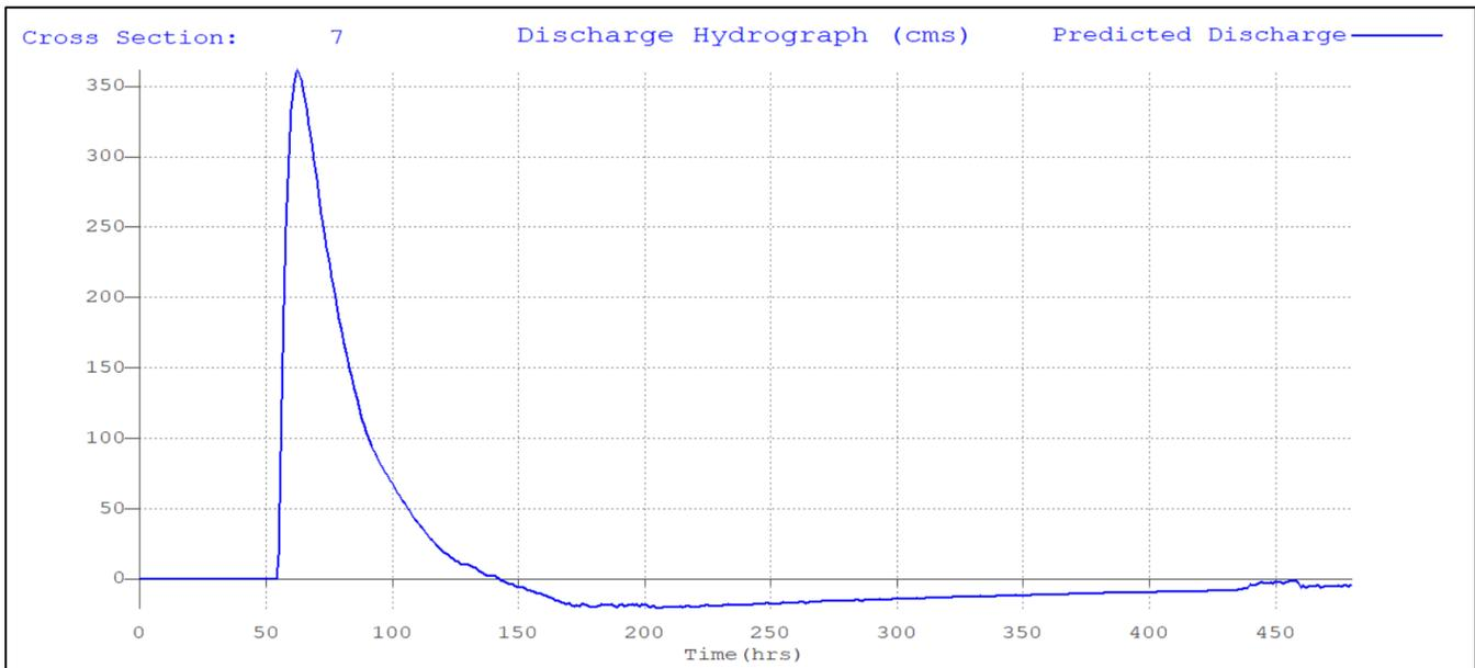
**A 22: Hydrograph at the cross-section below Lake Palmer, WA showing the debris flow into the lake around hour 60-70, followed by the outflow of the displaced water back downstream into the Similkameen River, as denoted by the negative flows from hour 150 onward. Default 40% breach scenario for the permitted CMM TSF.**
