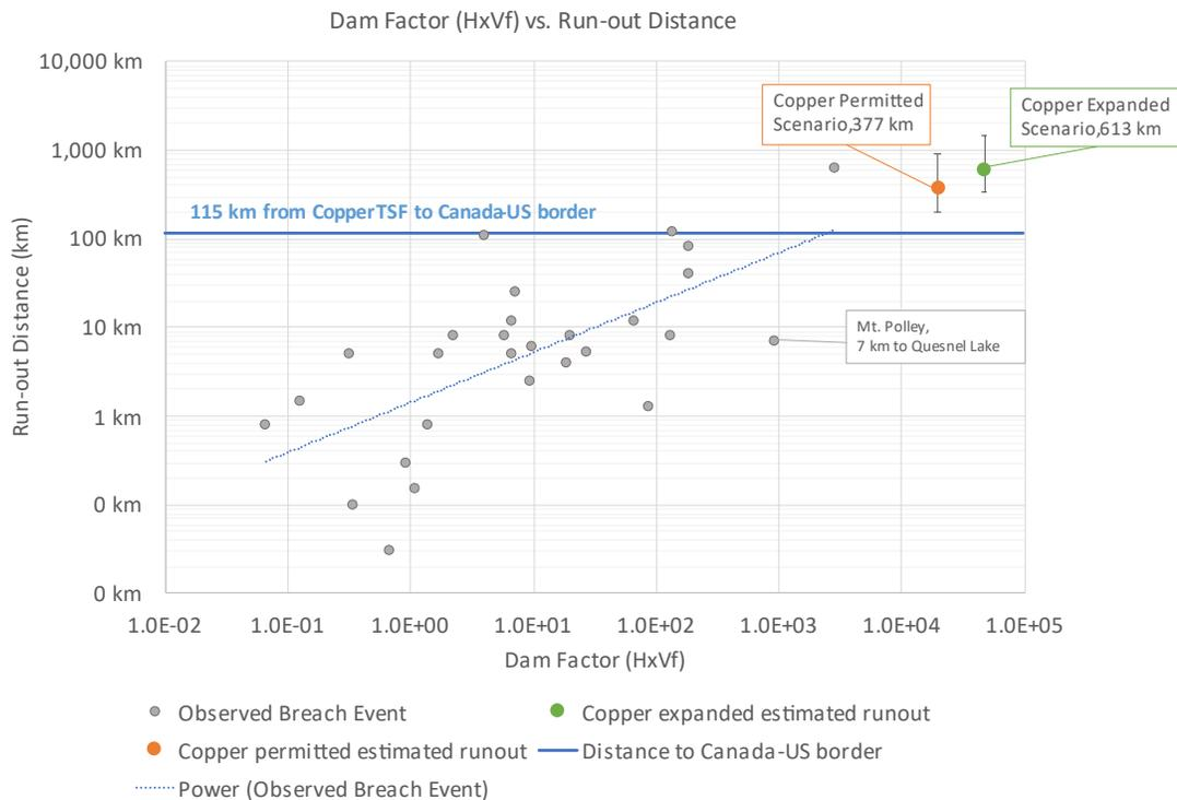
**Figure 2-3. Comparison of dam factor and observed breach run-out distance for historical breach events (historical breach data obtained from Larrari & Lall, 2018) and the estimated Copper TSF run-out distance. Blue horizontal line shows distance to US-Canada border for reference. Note that the Mount Polley runout distance was terminated by a downstream lake.**
