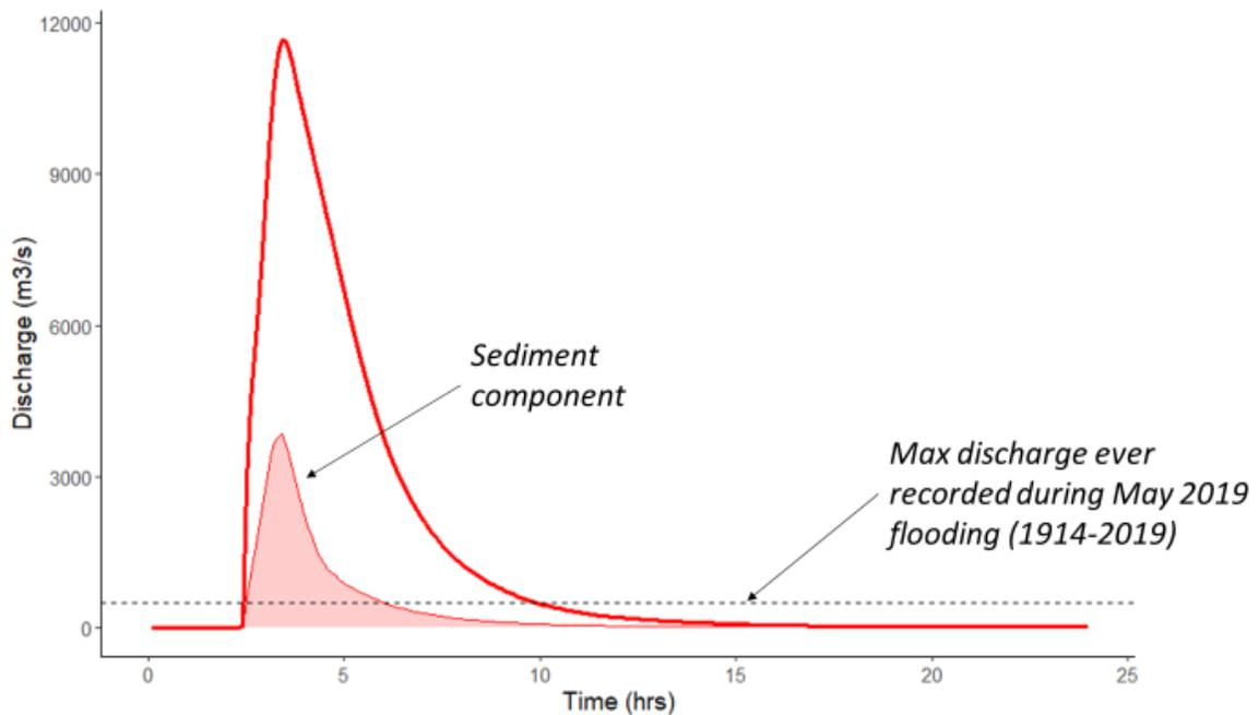
Figure 4-4. Timeseries hydrograph of the first 24 hours of the default permitted dam breach scenario. The bulked component (sediment and water; dark red line) is 12 times more than the maximum discharge ever recorded at gage 08NL007.
