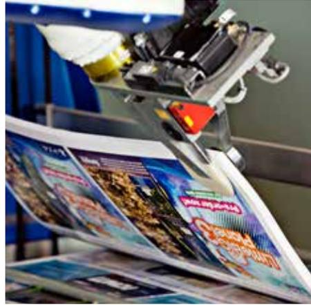
*Yaskawa Levanto separates, airs and moves a ream of sheets from a pile to a vibration table. This releases the operators Johnny Larsen and Jan Erik Grandahl from this heavy work.*
