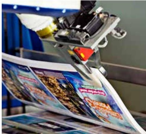
Yaskawa Levanto separates, airs and moves a ream of sheets from a pile to a vibration table. This relieves the operators at Stibo Graphic AS in Denmark, Johnny Larsen and Jan Erik Grandahl from this heavy work.
