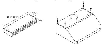
Secure the recirculating kit with the provided screws. Once secure, begin tightening each screw until the recirculating kit is flush with the range hood.
