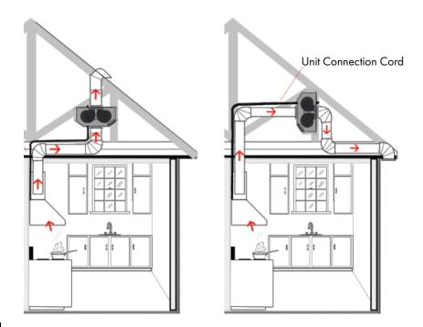
The Remote Blower is designed for our Remote Range Hoods. This unit is installed remotely in the interior of your home. This provides venting, but with reduced noise.
