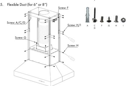
NOTE: Wall range hoods with single motors will come with a square to 6" round transition piece and will include a back draft damper. The ducting with these range hoods is 6". Dual motor wall hoods will come with a square to 8" round transition piece without a back draft damper. The ducting with these range hoods is 8" in diameter.
