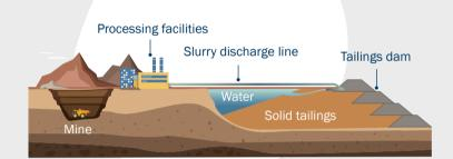
Many factors need to be taken into account when considering an option such as a tailings dam, including site geology, topography, soil conditions, earthquake or seismic risk, climatic conditions, environmental, social and cultural setting, the nature of the tailings and legacy provisions. Some tailings disposed of on land can produce acid and release heavy metals if exposed to oxygen – a process which cannot occur underwater.
